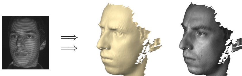
Figure 7: The surface generated from the image in Figure 3. Luminance values of stripe pixels in the original image were used to create a texture map.
