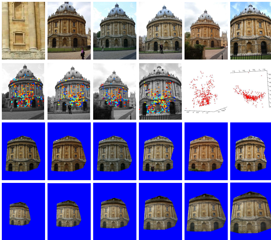
Figure 1: What information can be obtained from a visual query. Top row: The user provided query is shown in the top left image and is used to automatically retrieve images of the relevant building using a visual search engine [2]. Second row: robust 3-D feature and camera reconstruction is done in projective space. Here the projected 3-D features in some input views and affine reconstruction of the 3-D points are shown. Third row: Input views are used to render multiple novel views for each point of view in the projective space. These novel views have occluding objects and varying illuminations. Bottom row: Novel views based on different input views are fused together to remove occlusion and artifacts and render the scene with controlled illumination.
