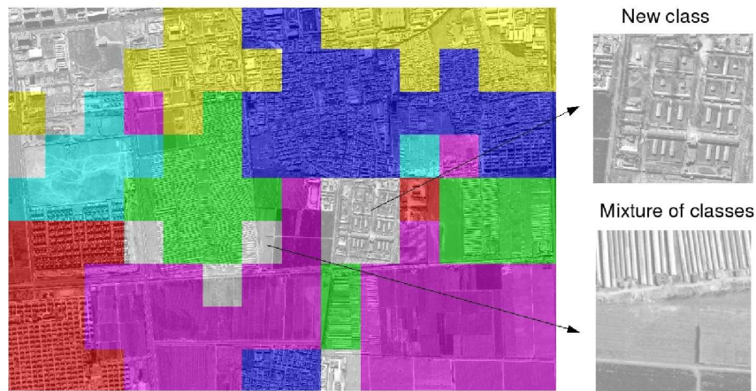
Figure 4: Classification results on a Quickbird image of size 2250 \times 3500 pixels. Each color corresponds to a class; white colour indicates the rejected patches.
