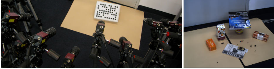
Figure 5: Setup of the real experiment. Left: the multi camera system observing the pattern for the Zhang calibration, right: the scene (image from the sixth camera).
