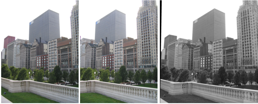
Figure 6: The two left images ( 1536 \times 2048 , \approx 40^\circ field of view) have been taken with a digital camera which purely rotated. An estimate of the rotation was given within 1^\circ accuracy, from which an infinite homography could be predicted. Given prediction and uncertainty the homography has been optimised and the resulting parameters have been used to stitch the images (right). The optimisation has been run upon 20 \times 20 samples only, distributed uniformly across the 3MPixel image. No heuristic smoothing or manual selection of a “good” pyramid level was applied. Note that this is an extremely challenging situation because of the frequency content. Remaining errors may be due to lens distortion, camera movement and changed illumination.
