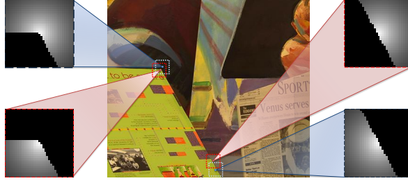
Figure 2: Computed adaptive support windows for four different pixels in an image. The brighter pixel means larger weight and the weights for darker region are close to zero.
