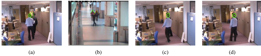
Figure 8: Examples of tracking failure. (a)(b) tracking multiple objects separately using the EM algorithm, (c) contour tracking with CONDENSATION, (d) mean-shift tracking with color histogram.
