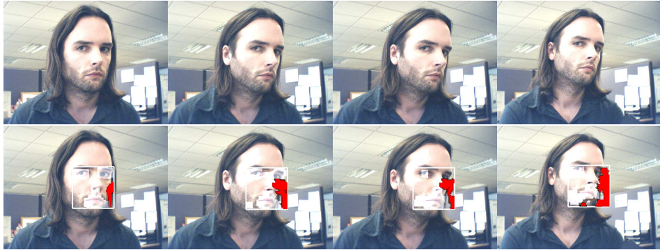
Figure 4: Feature selection under pose change. Large pose changes can lead to large regions of background being inside the target window. By labelling these as outliers, we avoid adaptation to the background. Row 1 shows input frames. Row 2 shows regions detected as occluded (red) and support regions of features (highlighted).
