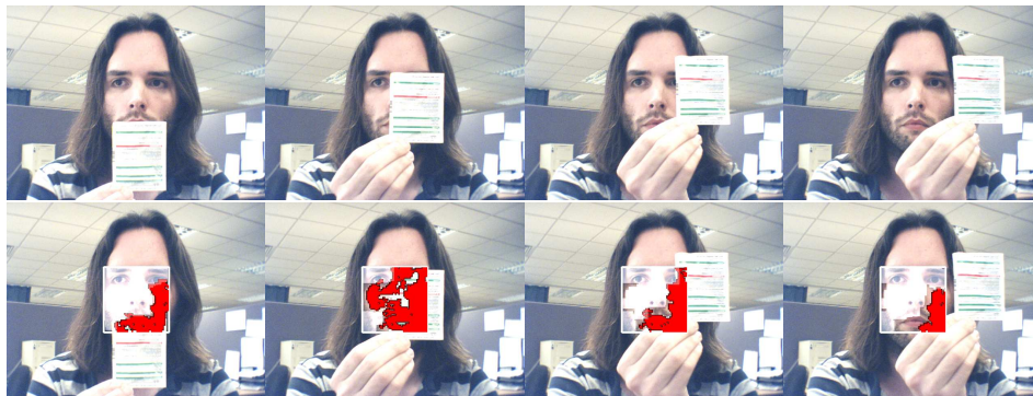
Figure 3: Online feature selection under occlusion. The model helps to avoid erroneous feature selection in the occluded regions. Row 1 shows sample frames. Row 2 shows regions detected as occluded (red) and support regions of features used in the classifier (highlighted).
