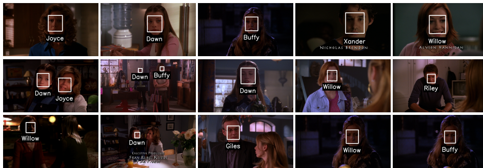
Figure 4: Sample identifications from episode 05-05. The top two rows show correctly matched faces, while the bottom row shows some sample failure cases. See text for details.
