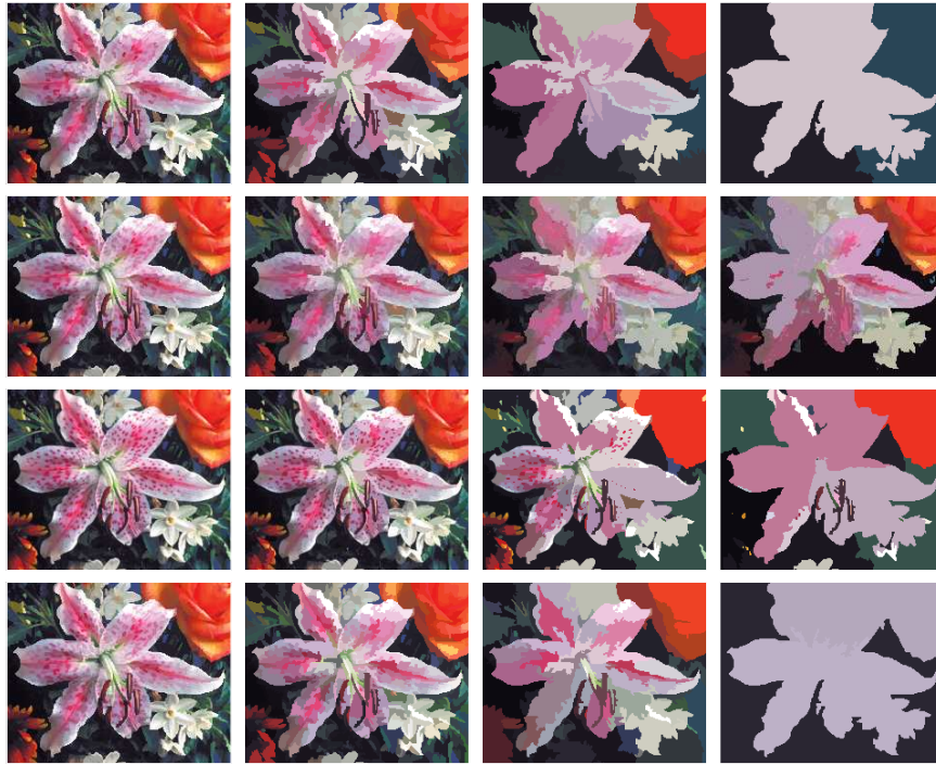
Figure 3: Colour sieve results for Lily test image using 8nn connectivity. Top to bottom: CCS, VAMOCS (openings only), VAMOCS (closings only) and VAMOCS (combined openings and closings). Left to right: area = 10,100,1000 and 10000.
