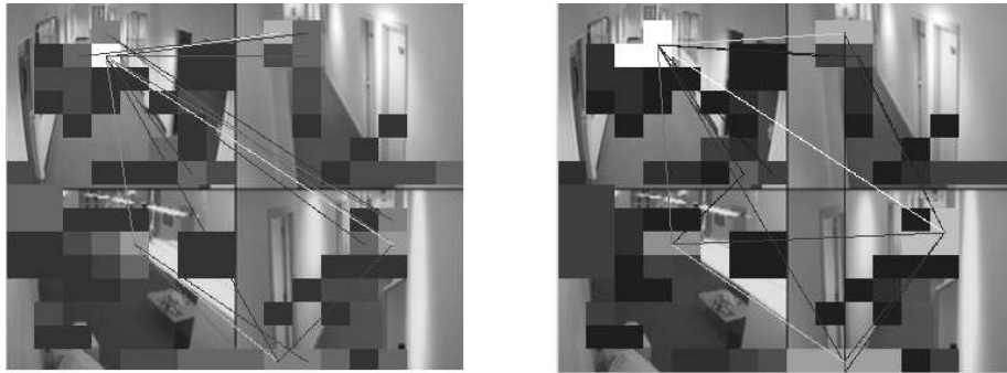
Figure 5: Left image shows the main identified entry/ exit blocks. Right Image shows the individual blocks that, if similar, are then recombined to form larger more populated blocks, shown by the constant colour areas.
