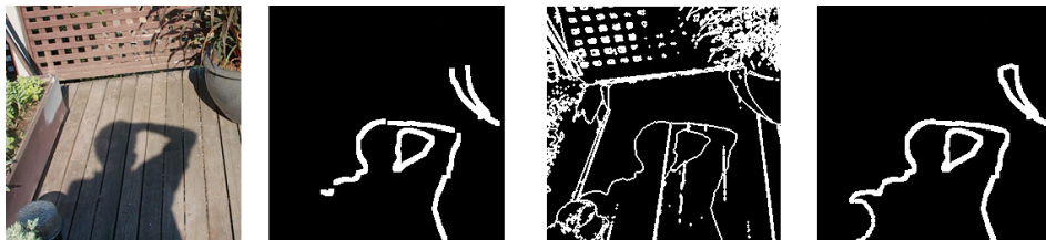
Figure 4: From left to right: the original image, detected shadow edges I_S , meanshift edges I_M and the resulting closure.
