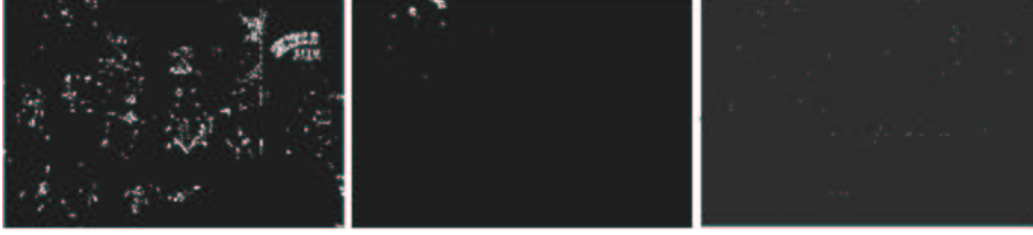
Figure 8. Detected dirt mask using spatial (left), temporal (middle) and multistage (right) median filtering.
