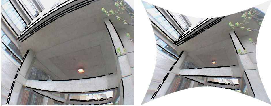
Figure 1: Image rectified using the rational function model. Edgels along 22 straight lines in the real world were detected in this single frame of video and the plumline constraint used to compute the distortion parameters.
