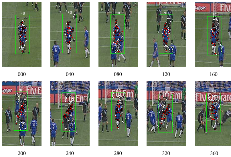
Figure 3: Tracking a soccer player. The images correspond from left to right and from top to bottom to every 40th frame of a 400 frame sequence. In each image, the red patches indicate the position of the model points, the white patches indicate the currently extracted points and the green rectangle represents the current region of interest.
