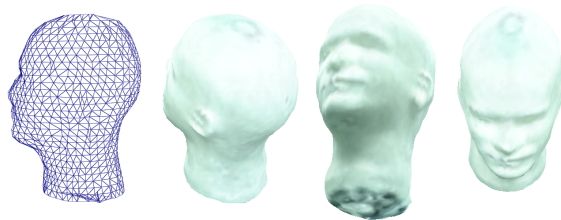
Figure 10: 3D model of the polystyrene head built from the estimated turntable motion.
