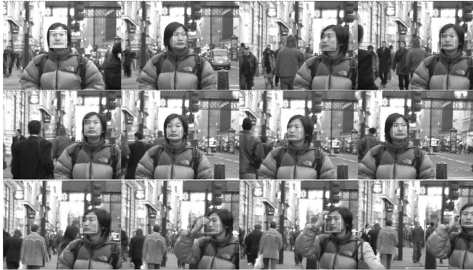
Figure 5: Experiment 3 - Tracking a partially occluded non-frontal male face in real-time with the proposed objective function. The figure shows example images from an outdoor sequence with a moving hand-held camera (Video Sequence 2).
