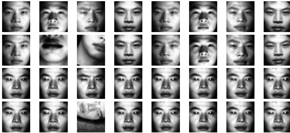
Figure 7: Resulting images after the histogram equalization is performed for manually and automatically registered ambient faces (top 2 rows) and for corresponding LED faces (bottom 2 rows). It is obvious that data from LED faces exhibits much less variation as compared to the data from ambient images. Bright pupils are prominent in the LED face data. There are localisation errors in some automatically registered faces.
