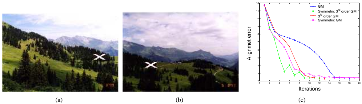
Figure 2: Registration results for projective motion. The initial estimate of the motion was given by the red X. The SGM converged better than the O3GM while the SO3GM showed the best convergence properties.
