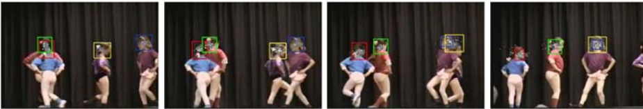
Figure 10: Tracking results for RealSeq3 . DPS fails to recover from occlusion for Object 4 - the girl with the black pants (frames 1,7,14,32 shown). (32 frames at 352x240).
