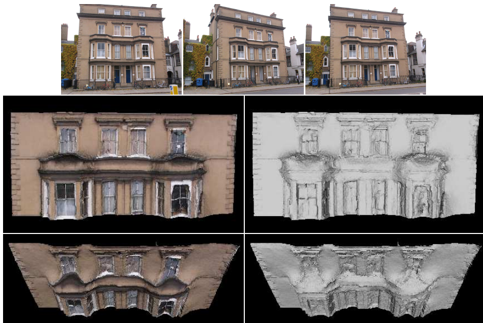
Figure 5: Building facade. Top: the images used. Bottom two rows, left and right: texture mapped and untextured relief surface. The base surface was the wall plane. The challenge of the scene is the shiny or transparent windows as well as the fine relief at places.
