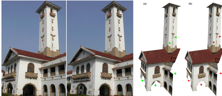
Figure 7: On the left are two images showing the initial vertex positions in green and the faired vertices in red. The faired vertices accurately correspond to corners and edges of the architecture. Notice the points along the archways, roof and balcony edges. The initial model and the EigenFaired model are shown in (a) and (b) respectively. The green and red arrows point out the presence and absence of modeling artifacts respectively.
