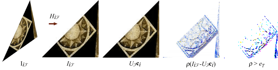
Figure 3: The triangular image patch I_{i\mathcal{F}} in the i -th image corresponding to face \mathcal{F} is warped to a fixed cell image I_{i\mathcal{F}} . The reconstructed cell image using the first five components of eigen-space is U_{\mathcal{F}}\mathbf{c}_i . The Geman-McClure norm between I_{i\mathcal{F}} and U_{\mathcal{F}}\mathbf{c}_i for \sigma=100 , and the spatial distribution of outliers ( e_T = \sigma/\sqrt{3} ) are on the right.
