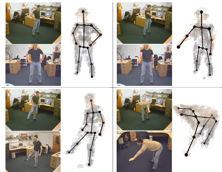
Figure 5: Examples of tracking for various body configurations. The reconstruction is performed from 4 camera views of which two are shown on the left. The displayed voxels' colours are the mean of the colours in all views. It can be noticed that shadows, cluttered environment and the self-occlusions lead to segmentation and reconstruction errors, which are mostly dismissed by the model matching.
