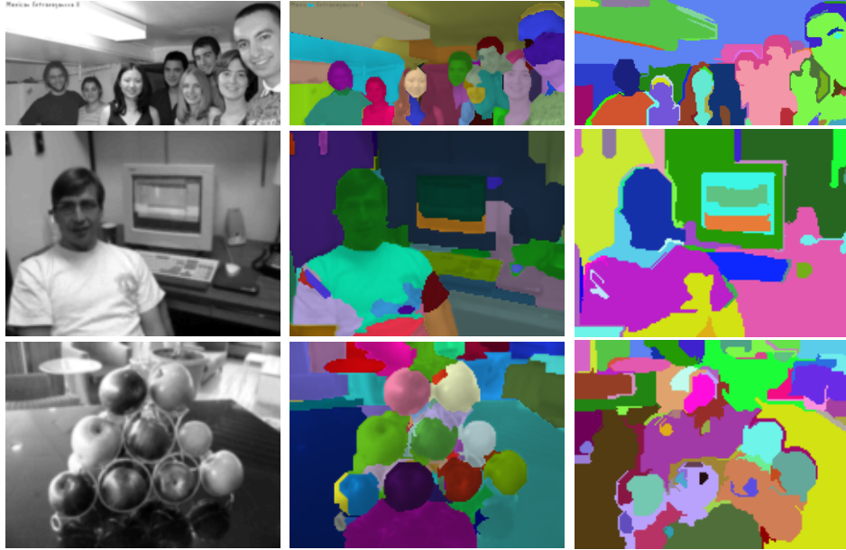
Figure 3: (Left column). Test images of indoor scenes. The top image is 239 \times 138 , and the two below are 160 \times 120 . (Center column) Segmentation results for our algorithm. (Right column) Segmentations using Felzenszwalb and Huttenlocher’s algorithm.
