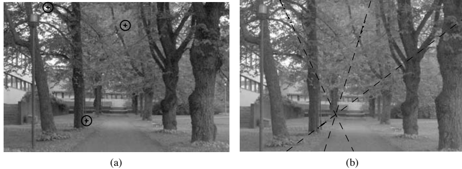
Figure 5: Behaviour of the epipolar line probability density when the epipolar geometry is known with a high level of accuracy. (a) Three randomly selected points in the first image. (b) One thousand independent samples, generated from each epipolar line probability density, lie in the vicinity of the mean epipolar line and show a large variation in disparity. The epipolar line corresponding to the point closest to the epipole in the first view is the most uncertain and the samples are more concentrated around the most probable point \mathbf{u}_2 on the line. The fundamental matrix and its covariance matrix were automatically robustly estimated from point correspondences as proposed in [1, 2].
