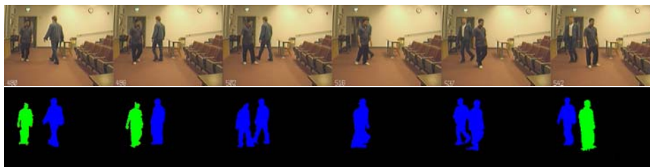
Figure 3: Select frames from tracking sequence. Two moving objects merge into a single blob (frame 502) and split (frame 542). The objects are color coded with BLUE corresponding to the first object and GREEN to the second one. The correct labels are restored after the merge-split sequence
