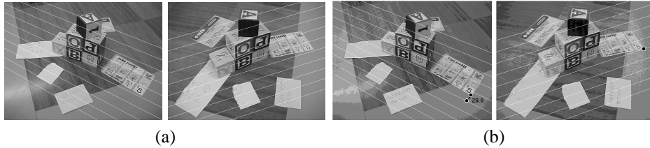
Figure 8: Test images, with an example of the epipolar geometry computed from perturbed pose. Points used to evaluate the fundamental matrix deformation are also shown.
