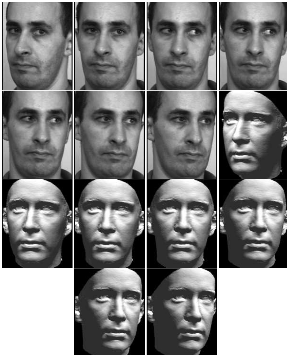
Figure 2: A short 7 image video sequence. Shaded reconstruction using all 7 images. The median deviation from a laser-scan of the same face is smaller 0.5mm.
