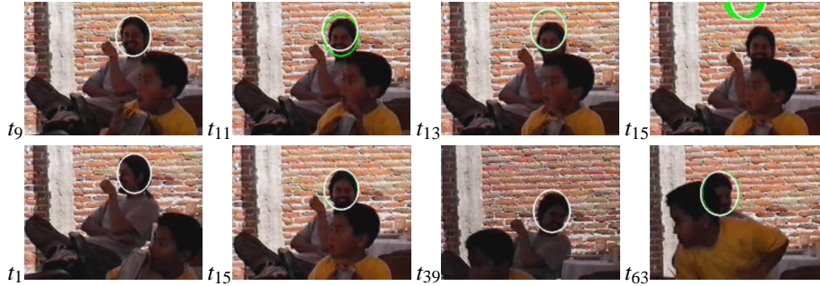
Figure 8: Head tracking 1 : top, shape tracker only. Bottom, shape+correlation tracker.
