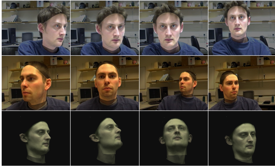
Figure 2: Example frames from successful tracks The morphable model is rendered overlaid on the target frame using the pose and model output from the tracker. Top and middle sequences were tracked using MI and Powell's method, the bottom using downhill simplex method and CR, a combination which offers better performance in controlled environment.
