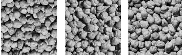
Figure 1: Three images of the same surface texture sample captured using different illuminant tilt angles.
