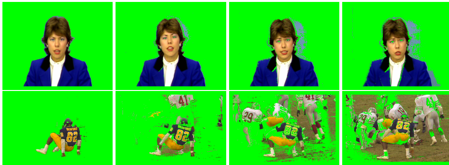
Figure 5: Segmentation Results using an adaptive Gaussian mixture model for the cif claire sequence (50 frames) and the more difficult cif football sequence (26 frames).
