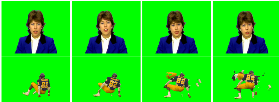
Figure 4: Segmentation Results using the proposed approach for the cif claire sequence (50 frames) and the more difficult cif football sequence (26 frames).
