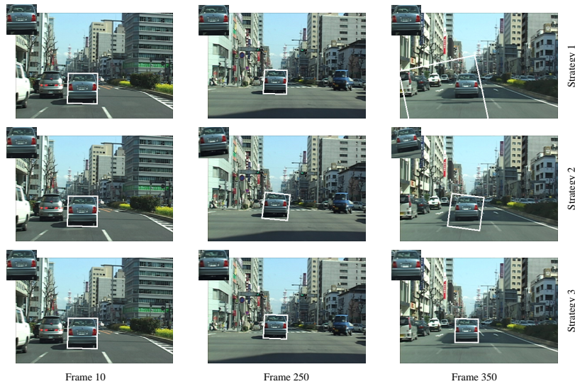
Figure 1: A qualitative comparison of update Strategies 1, 2, and 3. With Strategy 1 the template is not updated and tracking eventually fails. With Strategy 2, the template is updated every frame and the template “drifts”. With Strategy 3 the template is updated every frame, but a “drift correction” step is added. With this strategy the object is tracked correctly.
