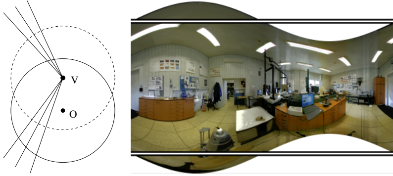
Figure 6: The X-slits mosaic camera has a blind spot (no light rays captured) depicted by the solid circle centered at O . When the viewer moves (simulated by moving the vertical slit V ), we have to rescale the resulting X-slits mosaic image in order to get correct aspect ratios. Black regions appear in the image at places we have no data. The white lines in the mosaic depict the original mosaic size.
