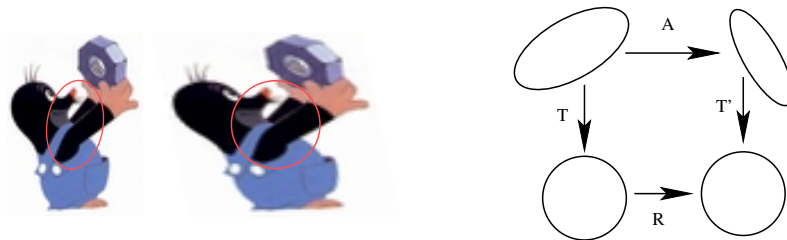
Figure 3: Picture of the Little Mole (left) and his normalised picture (middle). The covariance matrices are depicted as ellipses. The decomposition of affine transformation into two normalisations T , T' , and image rotation R (right).
