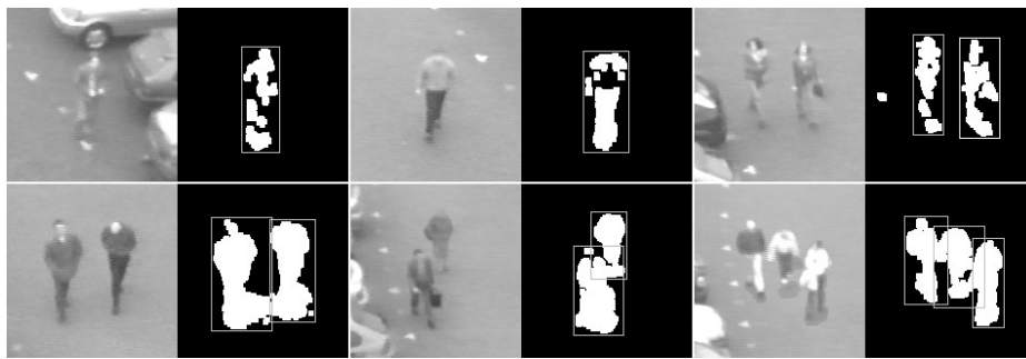
Figure 5: Fragmented (top) and merged (bottom) objects successfully disambiguated
