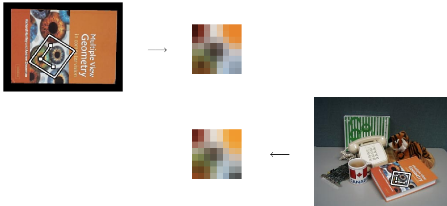
Figure 3: Extraction of affine invariant features from a pair of images. Groups of 3 interest points are used to calibrate the affine transformation to a canonical frame. The image region is then resampled in the canonical frame to form the feature descriptor.
