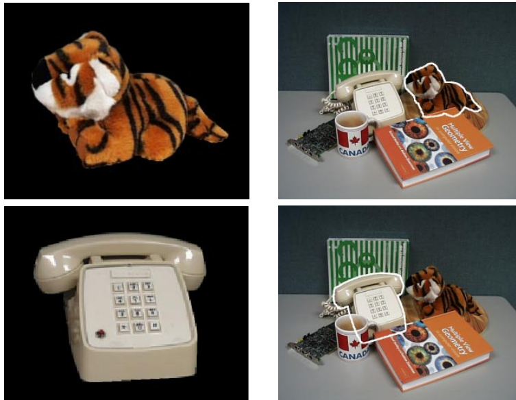
Figure 6: Object recognition using invariant features from interest point groups. The white outlines show the recognised pose of each object according to a homography. For 3D objects, this model is appropriate if the depth variation is small compared to the camera depth.
