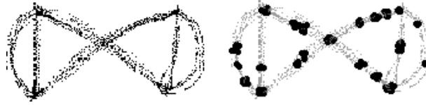
Figure 2: High density points extracted from a trajectory. The figure on the left represents the sequence of points. The centres of the circles on the figure on the right represents the selected nodes. The four corners where split and merge of trajectories occurs have been correctly identified as nodes.
