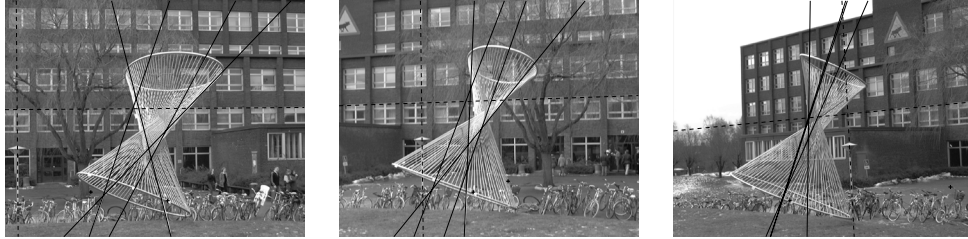
Figure 3: Three images used with the six lines and two points used in the reconstruction marked. The two dashed lines are the ones used to parameterize the problem.
