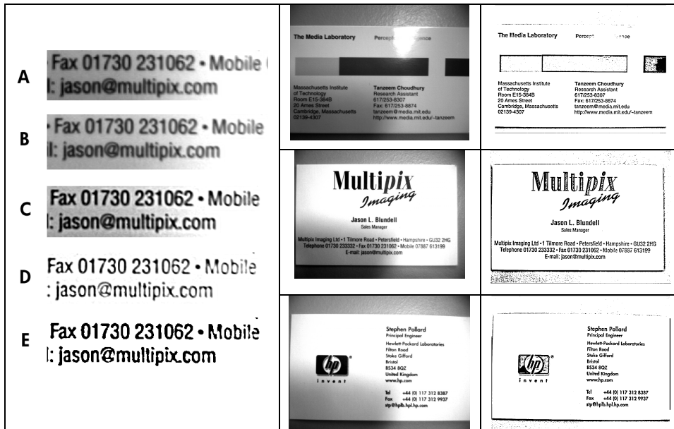
Figure 5. Left: Blowup of image portions showing all the stages that take the raw input image to the binary output. A: Demosaicked image; B: Upscaled image; C: After unsharp mask; D: After retinex-based filter (before thresholding); E: Thresholded binary output. Right: Three full examples showing the input images and the binary result from Section 4.
