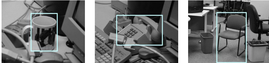
Figure 5: Examples of a detections of the mug, phone, and chair objects using a detector trained with fully labeled data.
