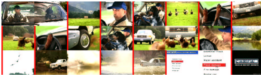
Figure 1: BIC keyframes generated by the browsing algorithm. The video sequence is successfully segmented into its constituting shots, shown by the red lines. The keyframes shown are those suggested by the BIC criterion, and provides a concise summary of the video sequence, useful for indexing and retrieval.
