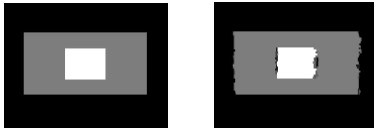
Figure 10 A comparison of the ground truth data and computed data (I) Left: ground truth disparity map, Right: disparity map using wavelets
