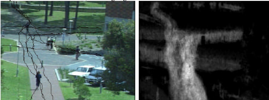
Figure 1a. Sample trajectories plotted in image plane and b) motion histogram image.
