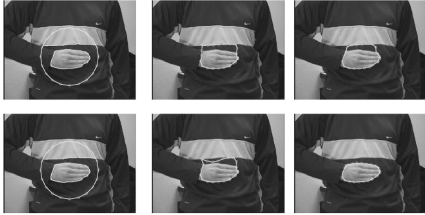
Figure 2: Results obtained with Snake potential (top row) iterations 1, 7, 20 and with adaptive potential (bottom row) iterations 1, 7, 10.
