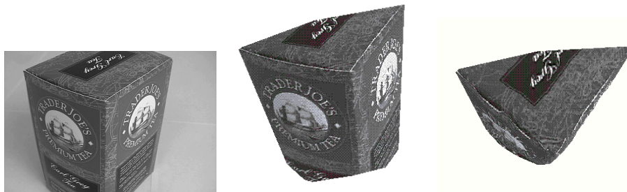
Figure 4: Reconstructed model of a Linux box based on 11 frames and 220 tracks. The average disparity is about 0.9 pixels per frame
