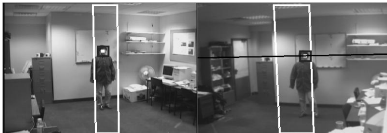
Fig. 1. Two views from the left and right cameras. A subject with face box, face box centroid (white dot), associated VA (big white box) (see Fig. 2). The epipolar line (black in right) is computed from the face box centroid of the subject in the left view.
