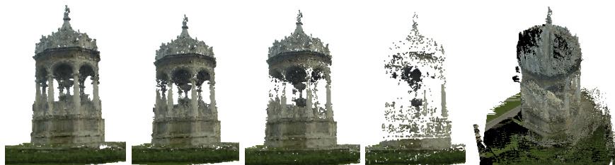
Figure 2: Results from the existing Space Carving algorithm using different threshold settings. The voxel array size was 128^3 , and the thresholds were 48,32,24,16 (of 255) respectively. Notice how much of the shape was obtained from the occluding contour (left).
