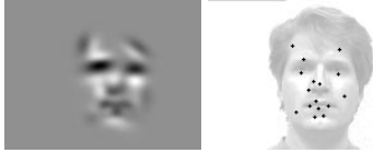
Figure 2: The images show a Gabor wavelet network with N = 16 wavelets after optimization (left) and the indicated positions of each single wavelet(right).
