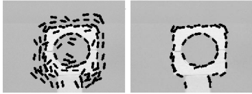
Figure 3: The figure shows images of a wooden toy block on which a GWN was trained. The black line segments sketch the positions, sizes and orientations of all the wavelets of the GWN (left), and of some automatically selected wavelets (right).
