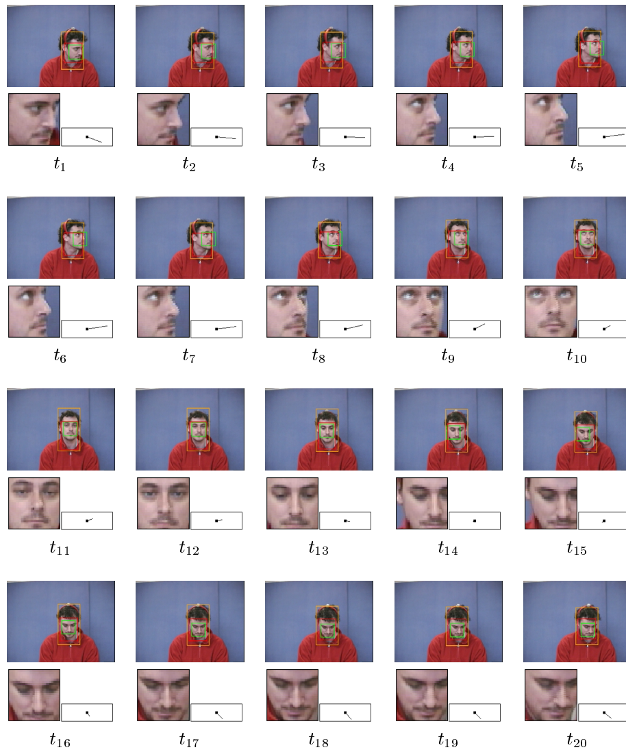
Figure 5: An example of continuous face position alignment and pose tracking over time. Each frame shows the whole image (top), the cropped tracked face (lower-left), and the tracked head pose (lower-right).
